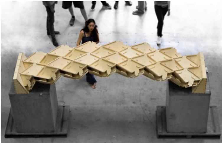
Fig. 4 Prototype assembled only with through tenon joints
