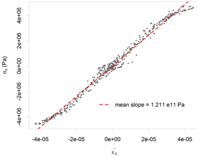
Fig. 11: Circumferential stress vs. circumferential strain during the transient test CSP03.
