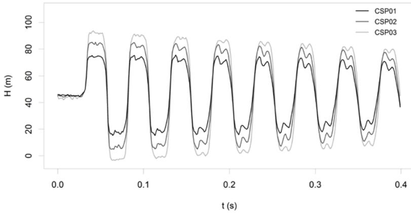
Fig. 2: Measured pressure data at the downstream boundary location for the waterhammer tests carried out at the straight copper pipe.
