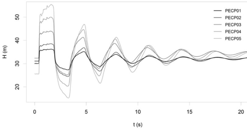
Fig. 8: Measured pressure data at the downstream boundary location for the waterhammer tests carried out at the polyethylene coil pipe.
