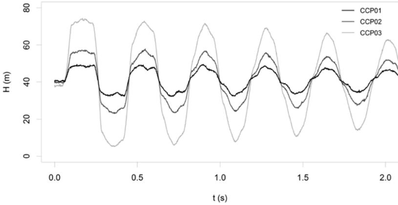
Fig. 5: Measured pressure data at the downstream boundary location for the waterhammer tests carried out at the copper coil pipe.
