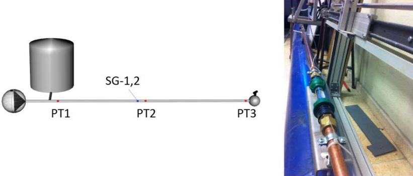
Fig. 1: Simplified schematic and view of the copper straight pipe.
