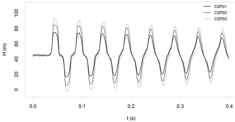
Fig. 3: Measured pressure data at the midstream boundary location for the waterhammer tests carried out at the straight copper pipe.
