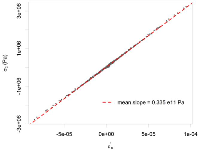
Fig. 12: Circumferential stress vs. circumferential strain during the transient CCP03
