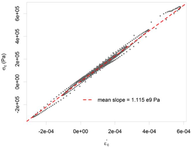
Fig. 13: Circumferential stress vs. circumferential strain during the transient test PECP03.
