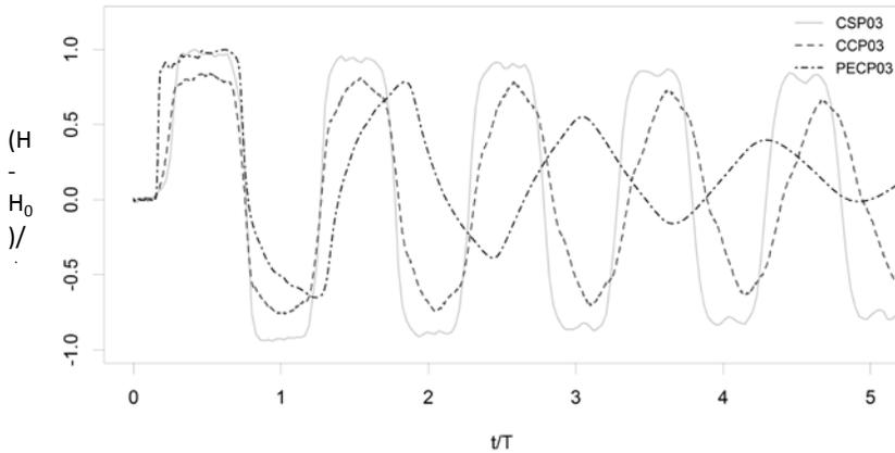
Fig. 10: Dimensionless transient pressures in the three set-ups.
