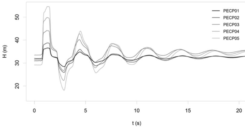
Fig. 9: Measured pressure data at the downstream boundary location for the waterhammer tests carried out at the polyethylene coil pipe.
