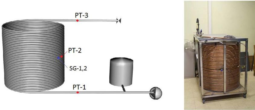
Fig. 4: Schematic and photograph of the copper pipe coil facility.
