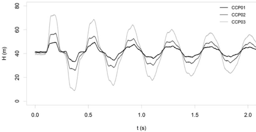
Fig. 6: Measured pressure data at the midstream boundary location for the waterhammer tests carried out at the copper coil pipe.
