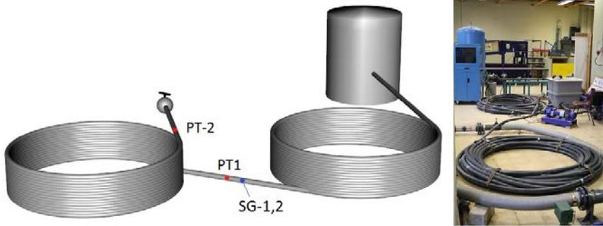
Fig. 7: Schematic and view of the polyethylene pipe coil facility.
