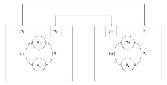
The above connectors connect the port  $p_1$  with  $q_2$  and the port  $p_2$  with  $q_1$ . Since they are all triggers, the connectors indeed describe the precise subset of interactions we wished to enable. However, if we look at the state machine of the system with the specified interaction model, some transitions that we wish to eliminate are still possible. Those transitions have been represented as dashed lines in the schema below.
