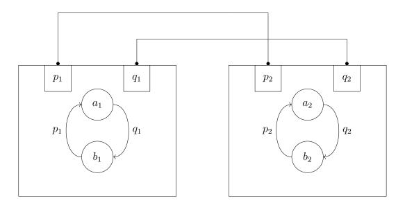
The above schema defines two connectors. The first one connects the ports  $p_1$  and  $p_2$  and the second  $q_1$  and  $q_2$ . Since all ports are given a synchron role, the only possible interactions are:
