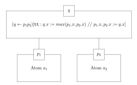
The connector specifies the possible interactions, in this case only one, and describes how data flows. As the task of describing interactions and associated data transfer policies can be very complex, the connectors in *BIP* are often hierarchically composed of multiple simpler connectors. For this reason, connectors, just as atoms, can export ports and thus be connected to other connectors.
