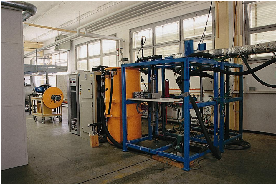
Figure 3: The experimental device at the thermodynamics laboratory of the EIVD. From the left to the right there is a refrigerating machine (with an ice generator), a storage tank and an apparatus with a horizontal insulated heat exchanger pipe mounted on the top. This pipe can be inclined in steps of 15°.
