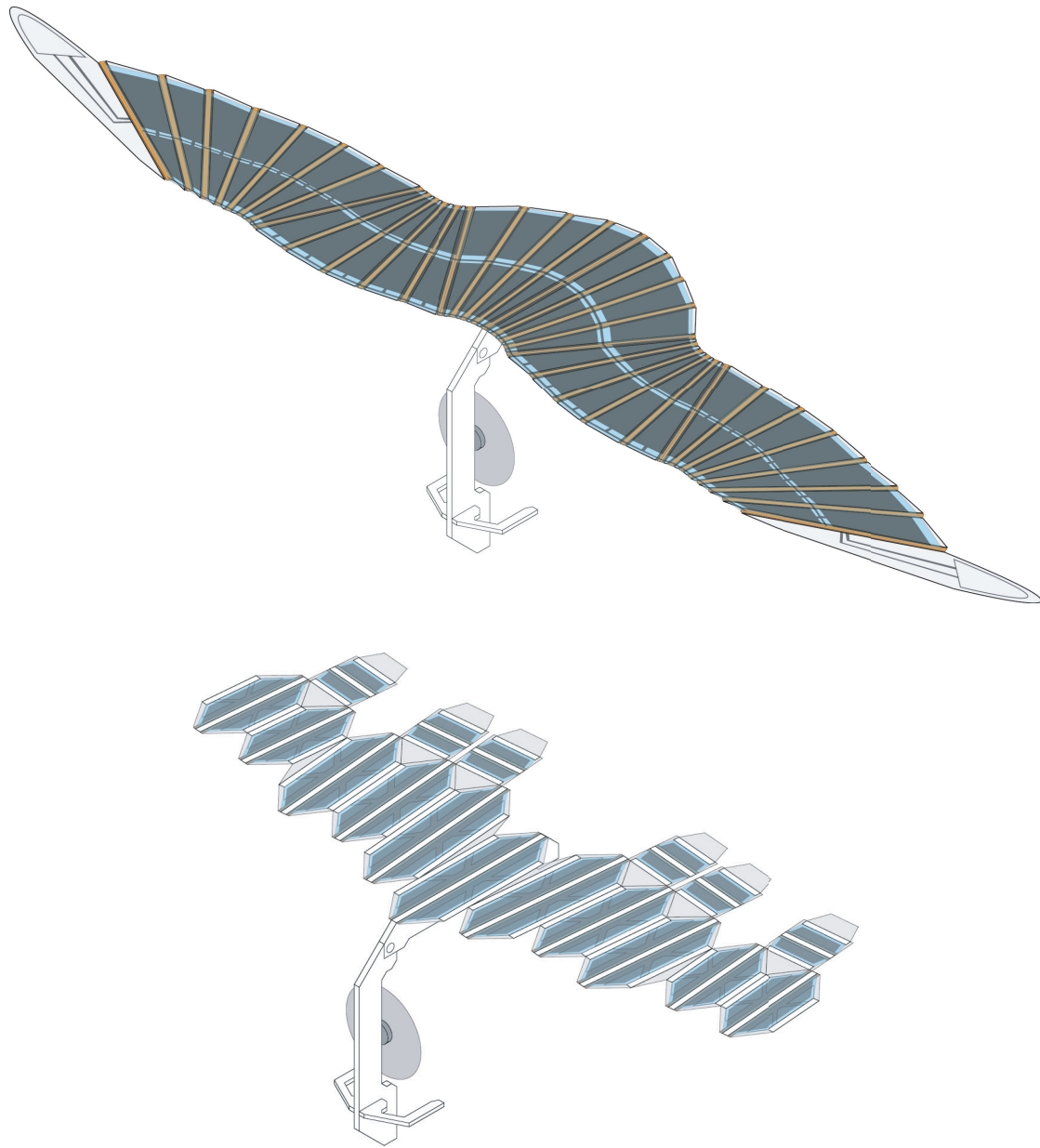
Figure D.6 – Other conceptual schematics of foldable MAV. The body has a role to protect the motor and hold the wing in the folded state.
