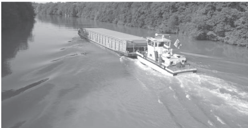
FIGURE 1. Pusher tug and barge on Rhone River, travelling upstream with approximately V_r = 4.2 m/s.
