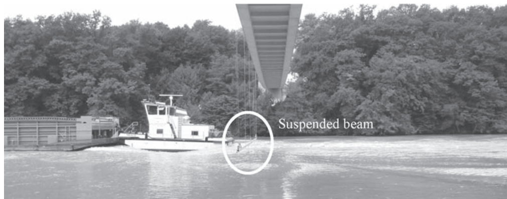
FIGURE 5. In situ test setup showing the suspended measurement beam below the bridge and convoy after passage, travelling upstream.
