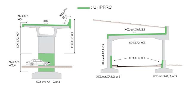
Figure 1: concepts of application of the local "hardening" of structures with UHPFRC.
