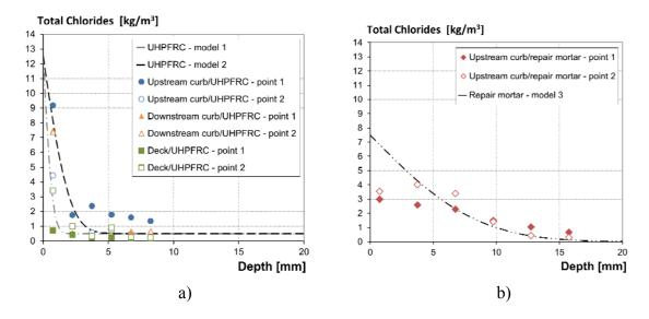
Figure 6: Chloride profiles after 10 years of exposure, bridge over river la Morge, a) UHPFRC, b) repair mortar applied in coring holes after 3 years exposure (age: 7 years), UHPFRC layer of 25 to 35 mm thickness over existing concrete.
