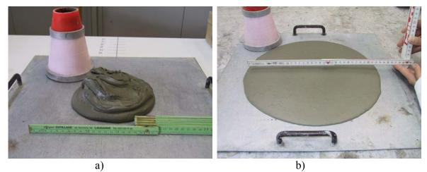
Figure 2: Mini-slump test results, UHPC mixes without a), or with b) blending with limestone filler.
