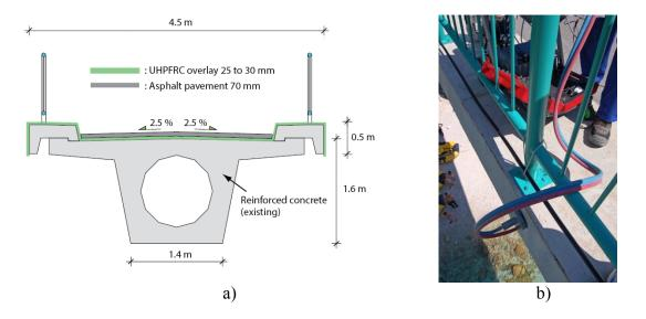
Figure 4: Application of UHPFRC. Log Čezsoški bridge – Soča river – Slovenia - July 2009, a) cross section of the bridge with concept of rehabilitation, b) air permeability tests after 2 years on lateral sides of curbs.
