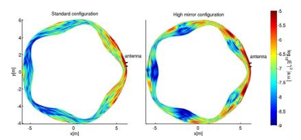
**FIGURE 2.**  $\log_{10}|E^+|^2$  for each configuration at the torus midplane. The black strokes show the antenna toroidal extension.
