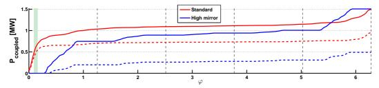
**FIGURE 3.** Cumulative (over toroidal angle) coupled power to the minority species over the whole (full lines) and the inner fourth (dashed lines) of the plasma volume for each configuration. The dashed lines shows each toroidal segment's limits and the green rectangle represents the antenna domain.
