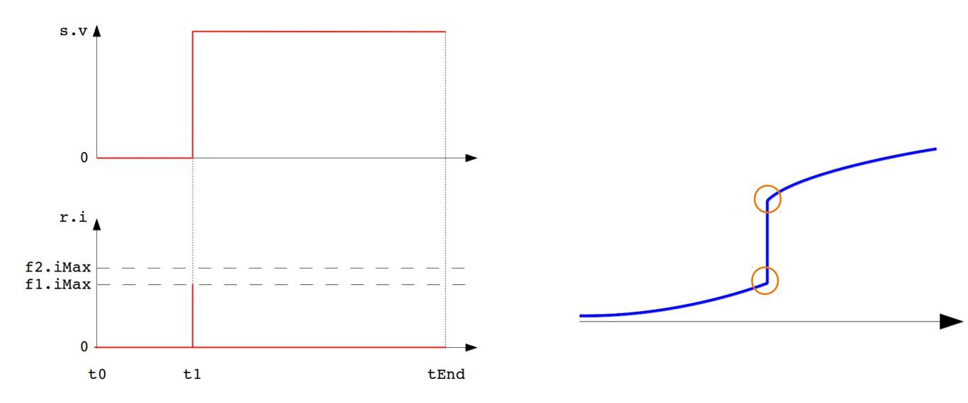
When the current reaches the rated value of the first fuse, this produces an input event, inverting the slope
