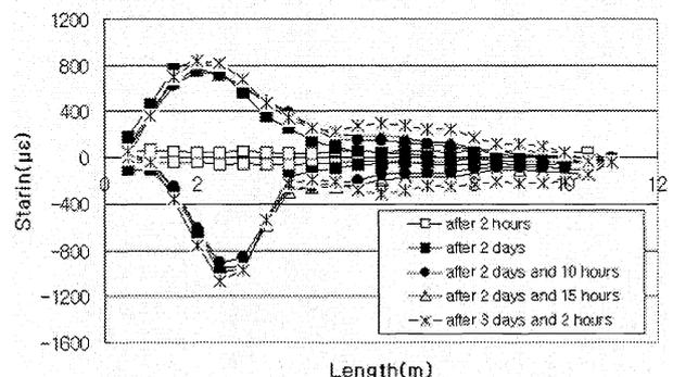
Fig 5 Distribution of strain along the smart reinforcing pipe for 2 fibres placed on opposite sides, showing a symmetric deformation. The deformation process stops after 2 days and remains steady.
