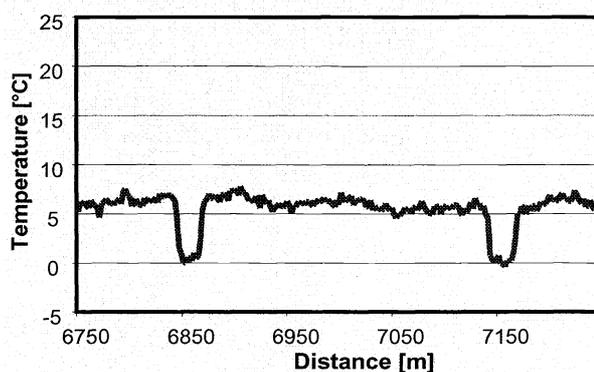
Fig 7 Temperature profile of a 500 m segment of the pipeline. Presence of splice boxes at air temperature (0 degC) is clearly observed. Any leakage would rise the temperature of more than 20 degC.
