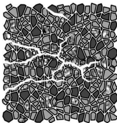
Fig. 1.1: A RVE at the moment of its ultimate failure.
