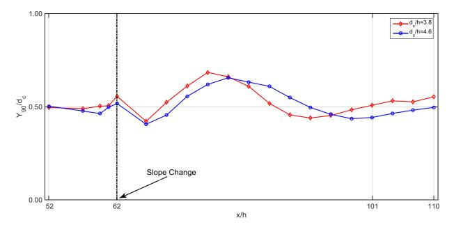
Figure 5 – Streamwise development of the normalized characteristic depth, for two unit discharges of  $0.35 \text{ m}^2/\text{s}$  ( $d_o/h=3.8$ ) and 0.46 m<sup>2</sup>/s ( $d_o/h=4.6$ ).
