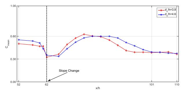
Figure 4 – Streamwise development of the mean air concentration for two unit discharges of 0.35 m<sup>2</sup>/s  $(d_o/h=3.8)$  and 0.46 m<sup>2</sup>/s  $(d_o/h=4.6)$ .
