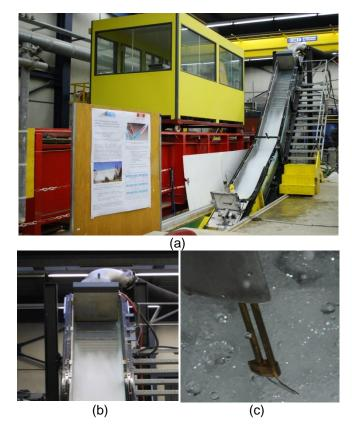
Figure 1 – Physical model of the stepped spillway with an abrupt slope change assembled at LCH-EPFL: a) General view; b) Initial reach of the chute and jet box, c) Dual fiber-optical probe in operation.
