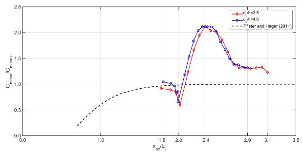
Figure 6 – Streamwise development of the mean air concentration ratio for two unit discharges of 0.35 m<sup>2</sup>/s ( $d_o/h=3.8$ ) and 0.46 m<sup>2</sup>/s ( $d_o/h=4.6$ ). The experimental data is normalized by  $C_{mean u}$ , upstream and downstream of the slope change (after Boes, 2000, and Takahashi and Ohtsu, 2012, respectively). At the slope change,  $x_{oo}/L_i \sim 2$  for both discharges.
