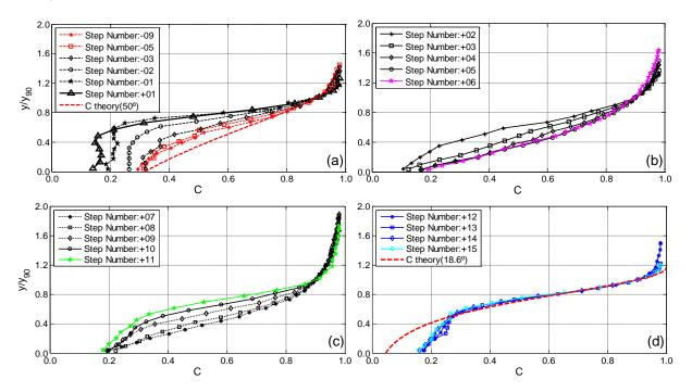
Figure 3 - Air concentration distribution upstream, downstream and along the slope change region ("-" and "+" signs represent the steps upstream and downstream of the slope change region, respectively (step numbers as per Figure 2): (a) sub-region I; (b) sub-region II; (c) sub-region III; (d) sub-region (IV):  $d_c/h$  =4.6. "C theory" was obtained from Chanson (1997), for uniform flow on a similar sloping chute, assuming  $C_{mean}$  equal to 0.6 and 0.3 for 50° and 18.6° slopes, respectively.
