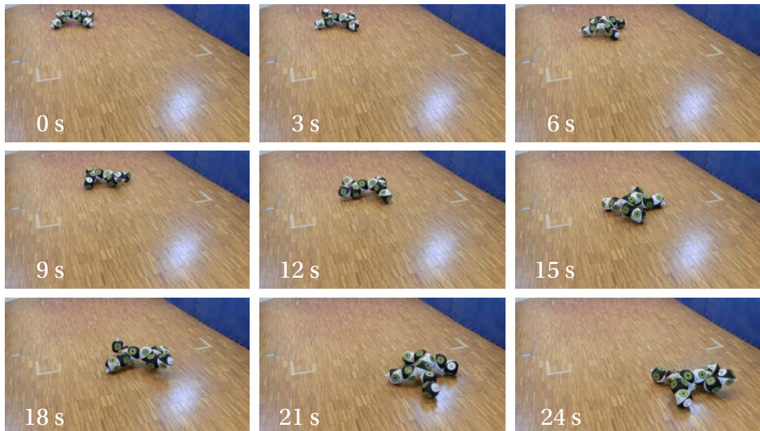
Figure C.1 – Locomotion of a quadrupedal structure made of five Roombots modules.
