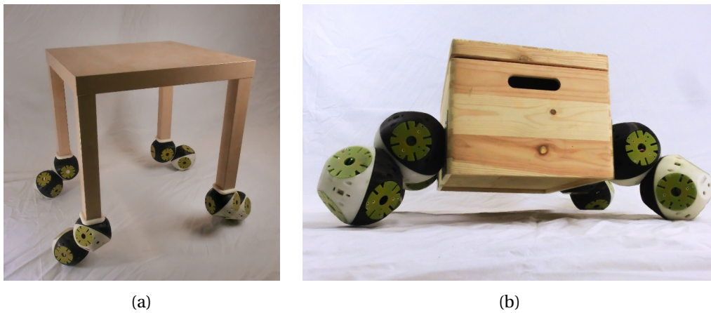
Figure 11.4 – Examples of standard pieces of furniture augmented with Plug-n-Play Robotic Elements: IKEA LACK table (a) and wooden box (b) equipped with four passive connection ports and four active Roombots modules connected to them.
