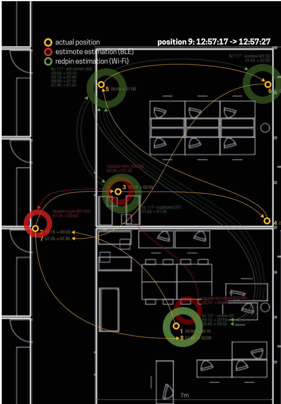
Positions 1-9 are existing Wi-Fi fingerprints made using the application. Sending interval is set to 5s. Estimate beacons are set to broadcasting power of 16dB (about 7m in range); there are 3 beacons at positions 1, 2 and 3
