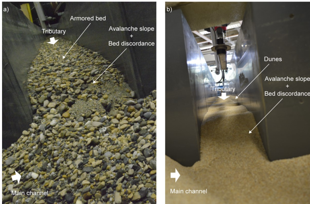
Figure 6.6 a) Tributary bed at equilibrium for Q_r = 0.11 with non-uniform sediments (set II). b) Tributary bed at equilibrium for Q_r = 0.11 with uniform sediments (set III).
