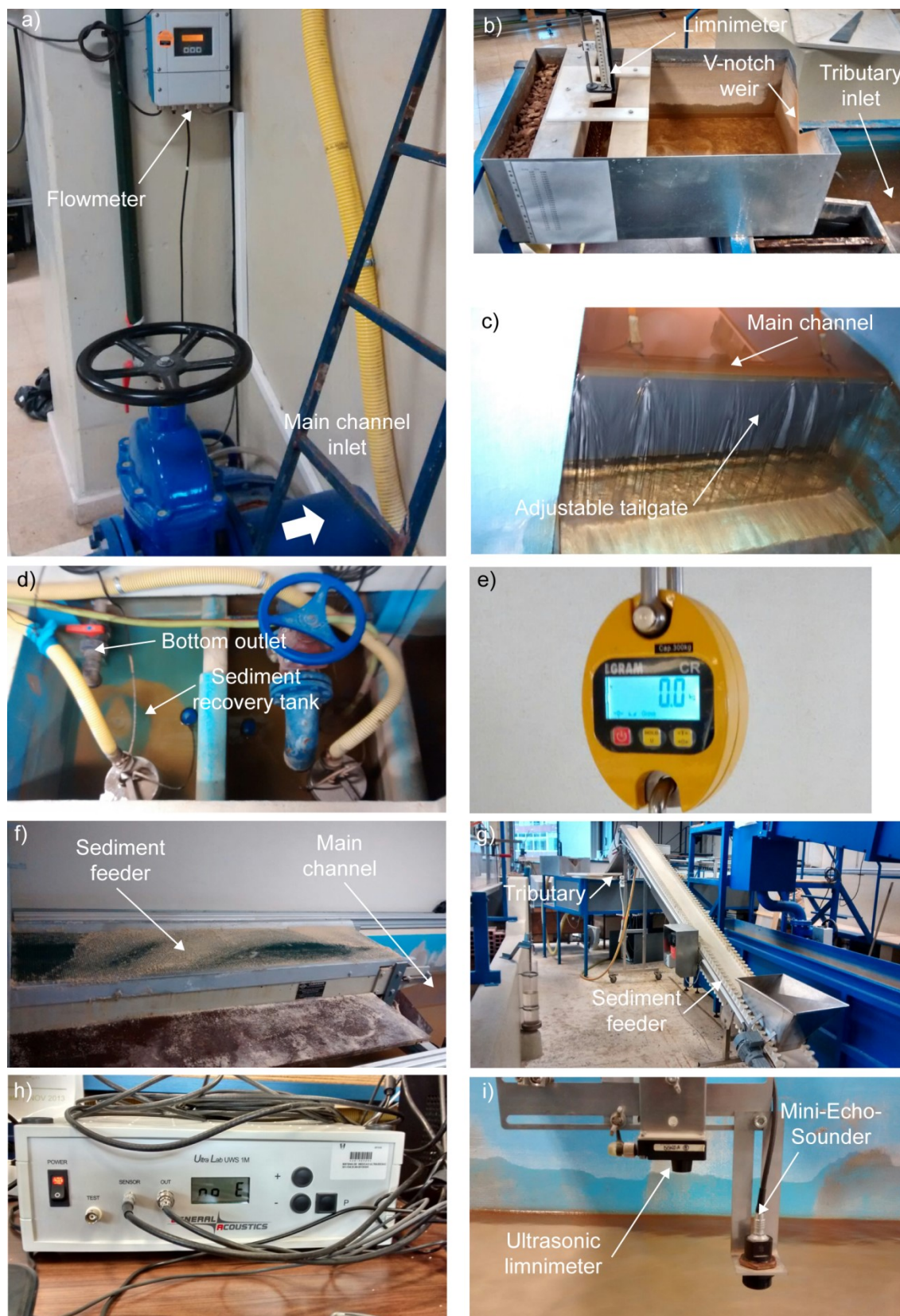
Figure 3.7 Measuring instrumentation and equipment of the experimental facility at the IST-UL. a) Electromagnetic flowmeter at the main channel inlet. b) V-notch weir at the tributary inlet. c) Adjustable tailgate at the downstream end of the main channel. d) Sediment recovery tank and bottom outlet. e) Digital scale. f) Sediment feeder of the main channel. g) Sediment feeder of the tributary. h) Acquisition data box of the Mini-EchoSounder. i) Ultrasonic limnimeter and MiniEchoSounder.
