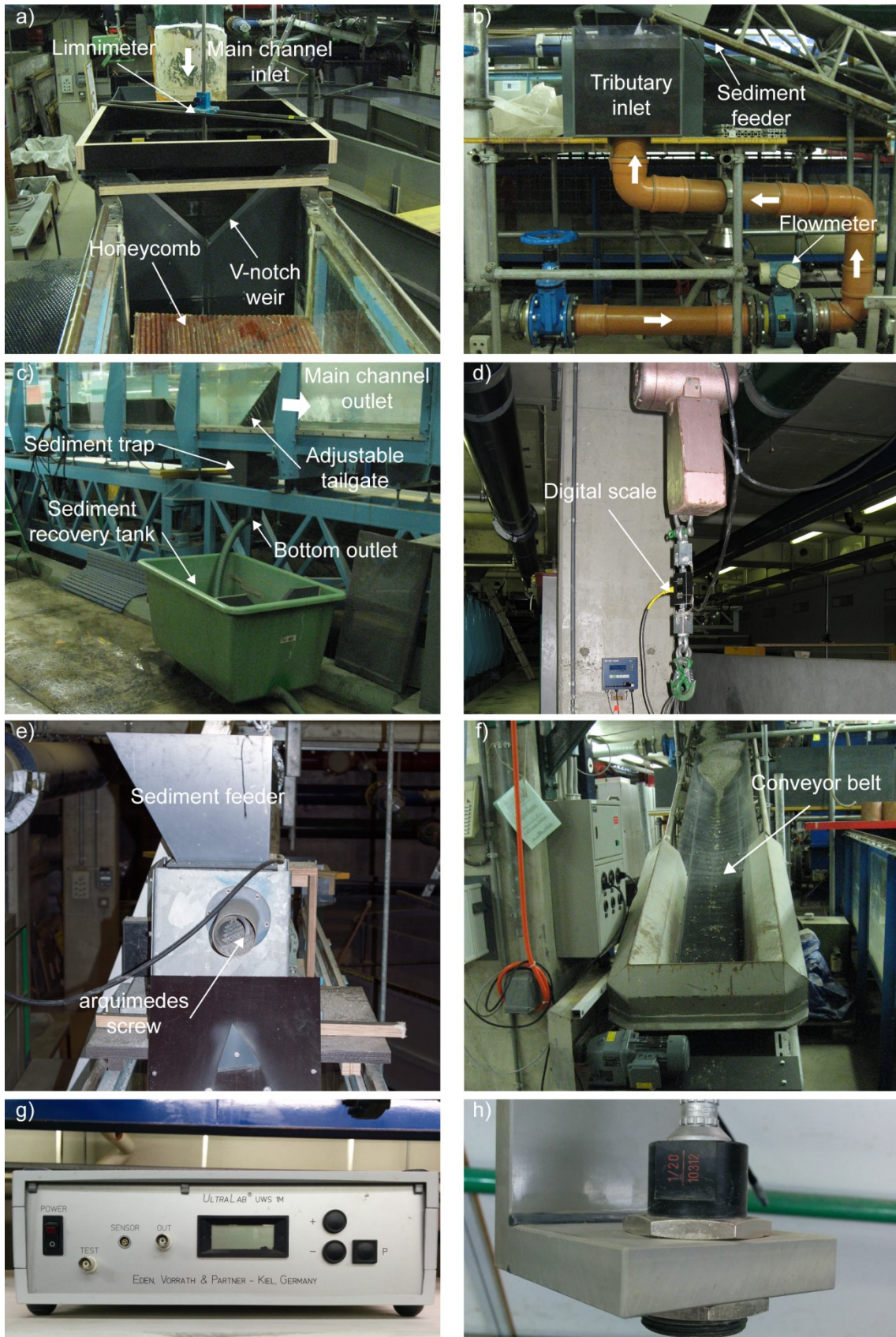
Figure 3.5 Measuring instrumentation and equipment of the experimental facility at LCH-EPFL. a) V-notch weir at the main channel inlet. b) Water supply system for the tributary. c) Sediment recovery system. d) Digital scale. e) Sediment feeder of the main channel. f) Sediment feeder of the tributary. g) Acquisition data box of the Mini-EchoSounder. h) Mini-EchoSounder probe.
