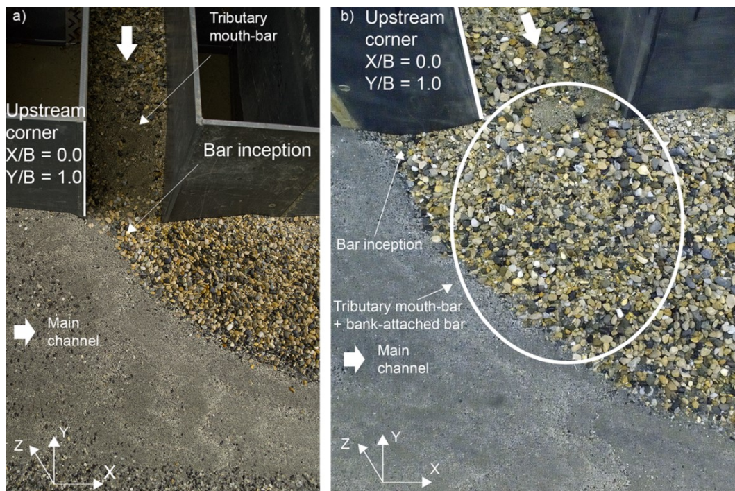
Figure 5.5 Perspective views of the tributary mouth at equilibrium corresponding to the low discharge ratio with a) \alpha = 90^\circ and b) \alpha = 70^\circ
