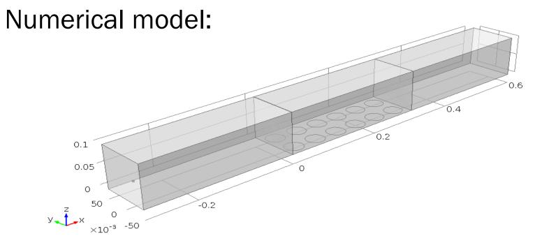
6x2 cells paving a duct wall
