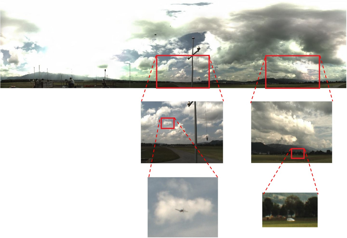
Figure 7.4 – Omnidirectional image obtained with the Giga-Eye system at 82.3 MP resolution. This omnidirectional image corresponds to one single frame of the 9.5 fps video obtained by the system. Flying plane and the moving car are shown in sub-windows
