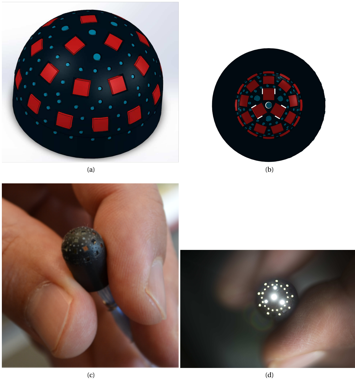
Figure 3.11 – The final mechanical design for the prototype, (a) and (b) Solidworks Drawings ,(c) and (d) the fabricated and assembled prototype
