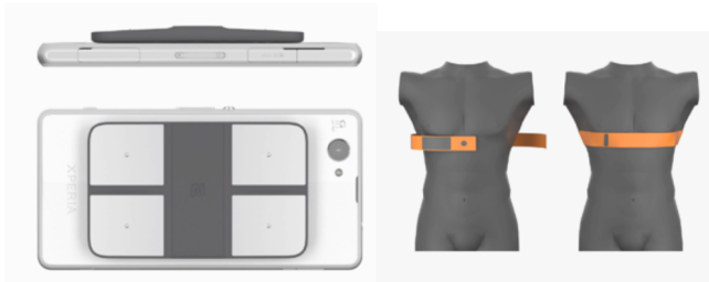
Figure 1. Device for physiological signal acquisition. Device can be attached behind a phone, and the metal pads touched by the user or can be attached using a chest strap.
