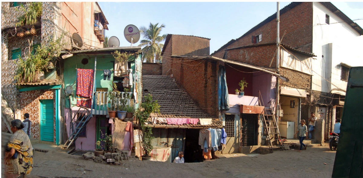
Photo 100. The house in the middle gradually disappears behind the rising street level. Both neighbors just keep up, while the higher buildings at both ends of the photo are ahead in the race. This part of Dharavi Main Road summarizes the phenomena mentioned in this chapter. December 28, 2012.
