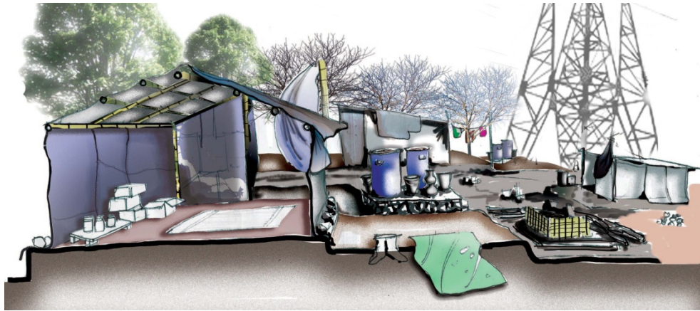
Drawing 10. Settling starts with a structure of bamboo poles and plastic tarpaulins. The main arrangement consists of segregating the dry part of the household (interior) from the wet part (exterior), as explained in Water (page 140). Image courtesy Sonam Ambe.
