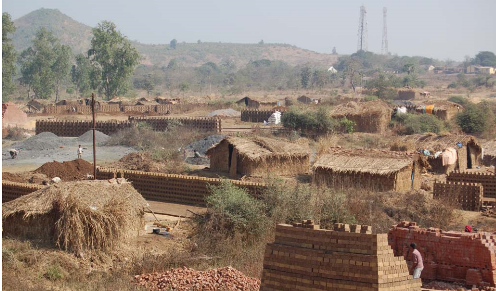
Photo 30. Clay-rich soil is typically found in riverbeds, which are only accessible during the dry season. Therefore, brick maker's houses are temporary and kacca . Near Manor, January 5, 2013.
