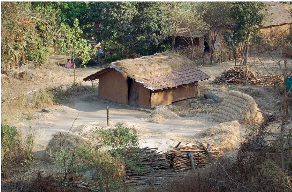
Photo 28. A house built of the materials that surround it. The only pucca are the ceramic roof tiles. The rice thath on top provides extra protection against the sun. Near Kelthan, January 18, 2013.
