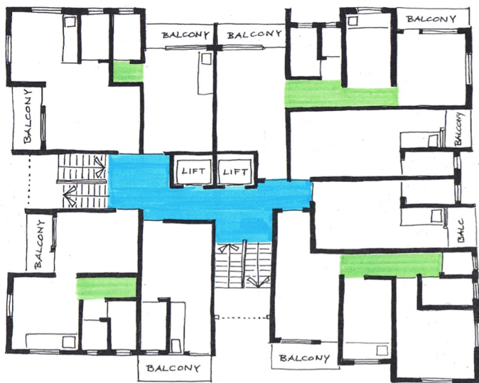
Drawing 33. In Rajgir Sadan, the hall (blue) typically does not afford the ordinary social life found in the street. This kind of single purpose circulation space is found inside the tenements as well (green).
