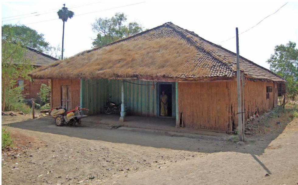
Photo 34. Mrs. Patil's kacca house two weeks before replacement with a brickwork-and-cement version. The neighbors already changed to pucca. Kelthan, January 18, 2013.
