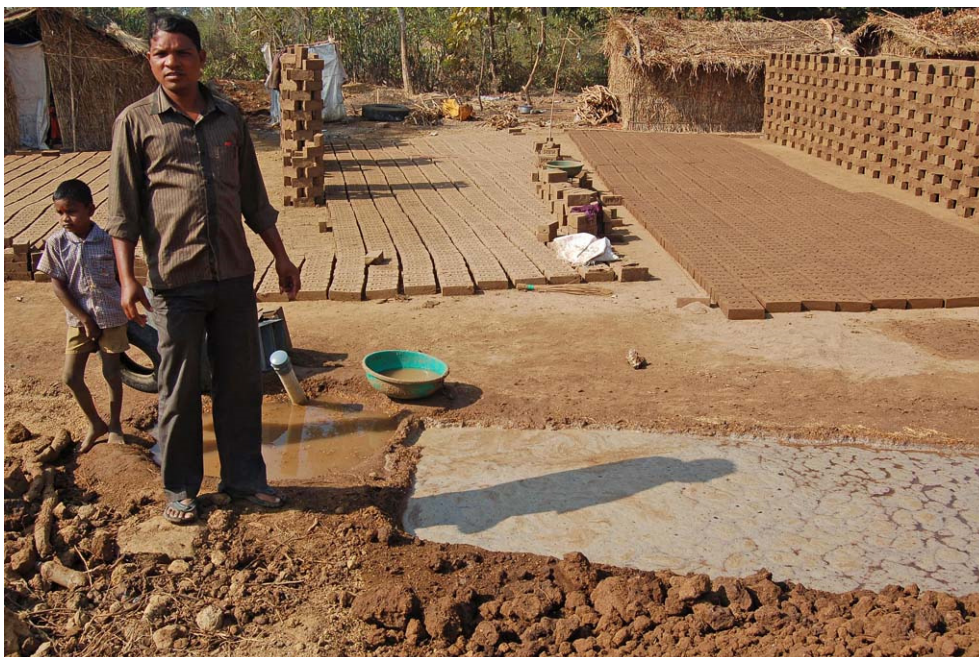
Photo 29. Brick making starts with molding clay-rich soil and drying the raw bricks for four days. Near Manor, January 5, 2013.
