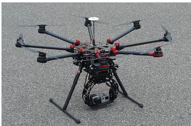
Fig. 9: IR-multi-copter drone of the PVLab
