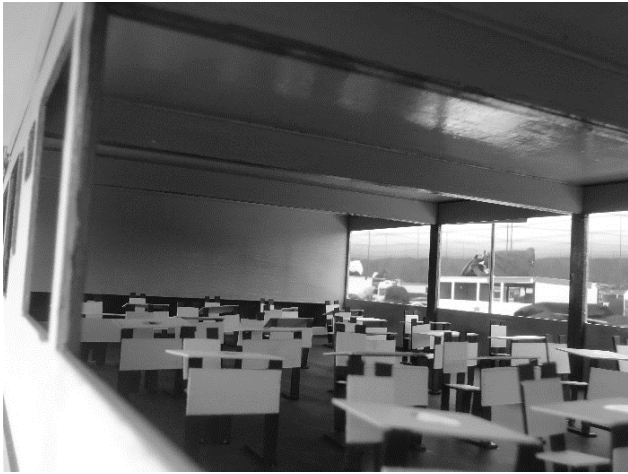
Figure 5: Internal View of the Scale Physical Model with an Anidolic System in the artificial sky
