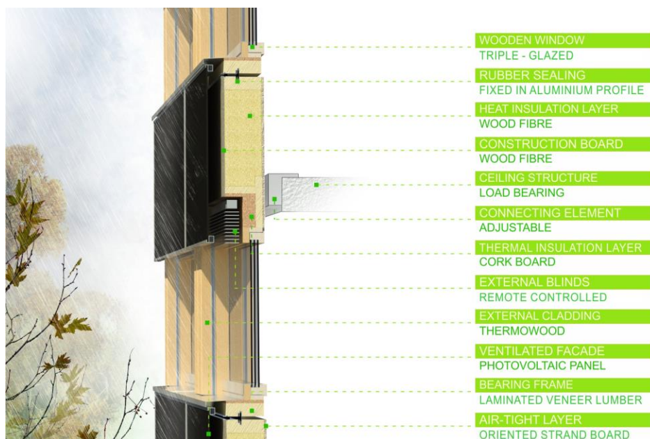
Figure 2: Typical composition of transparent panels.
