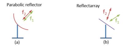
Figure 1.2: The advantage of a high-functional reflectarray antenna in a satellite communications' ground station. While the beam direction at different frequencies remains unchanged in a parabolic reflector, the multi-band performance of a reflectarray antenna allows wireless connection with several (here two) geostationary satellites in different positions at different frequencies (here  $f_1$  and  $f_2$ ).
