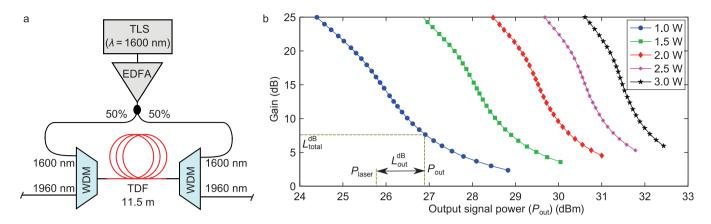
Figure 2 GU layout and characterization. (a) Layout of the GU consisting of 11.5 m of TDF. (b) Experimentally measured gain as a function of output signal power Pout. The output power of the laser  $P_{\text{laser}}$  can be estimated by taking into account the total losses of the cavity  $(L_{\text{out}}^{\text{IdB}})$  and the out-coupling losses  $(L_{\text{out}}^{\text{IdB}})$ . EDFA, erbium-doped fiber amplifier; WDM, wavelength division multiplexer.
