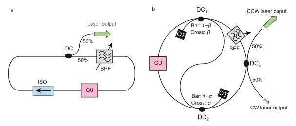
**Figure 3** Investigated fiber laser configurations. (a) Ring cavity and (b) theta cavity. The cross-coupling ratio of DC<sub>1</sub> can take values  $\beta = 10\%$ , 50%, or 90%. The cross-coupling ratio of DC<sub>2</sub> is maintained at  $\alpha = 10\%$ . OT, optical terminator.
