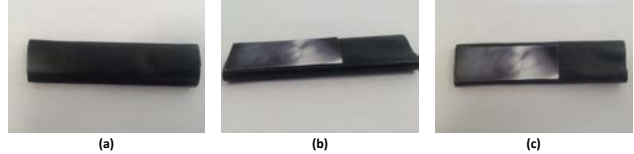
Figure 2: Example of the finger vein artefact (a) Back view (b) Side view (c) Top view
