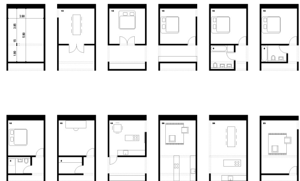
Fig 2: Functional module measuring 22m 2 adapting to the different functionalities of the accommodation
