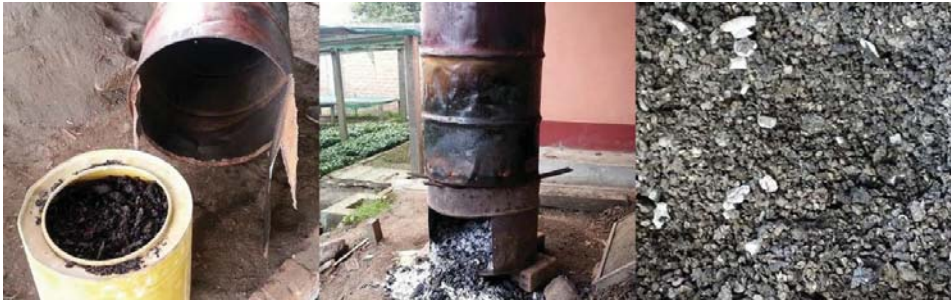
Figure 5 Simple Biochar production with a double cylinder oven
