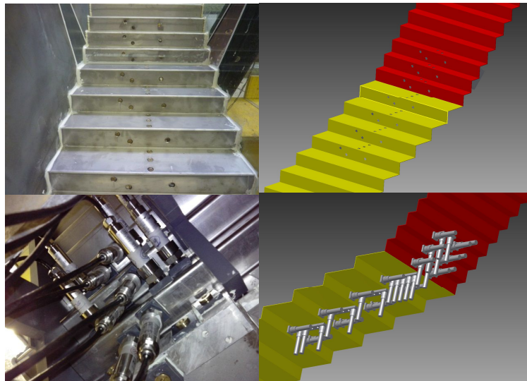
Figure 3. Pressure transducers installed in the vicinity of the slope change: photographs (left side) and schematics (right side) of the 50°-30° slope change equipped with pressure transducers.
