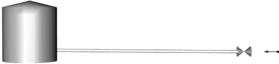
Figure 6. Single straight pipe with a free moving valve at the downstream end.
