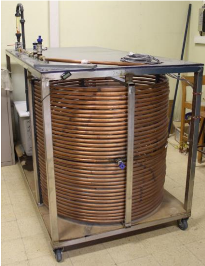
Figure 1. Picture (left) and scheme (right) of the copper pipe coil facility used during the experimental tests.
