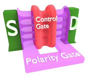
Figure 2.1 – 3D conceptual view of the proposed device. Source/Drain pillars supporting a vertical stack of nanowires are shown in green. The Gate-All-Around polarity gate, covering the side regions of the channel is shown in violet, while the central control gate is shown in red. The model is shown in proportion to the actual fabricated device dimensions.
