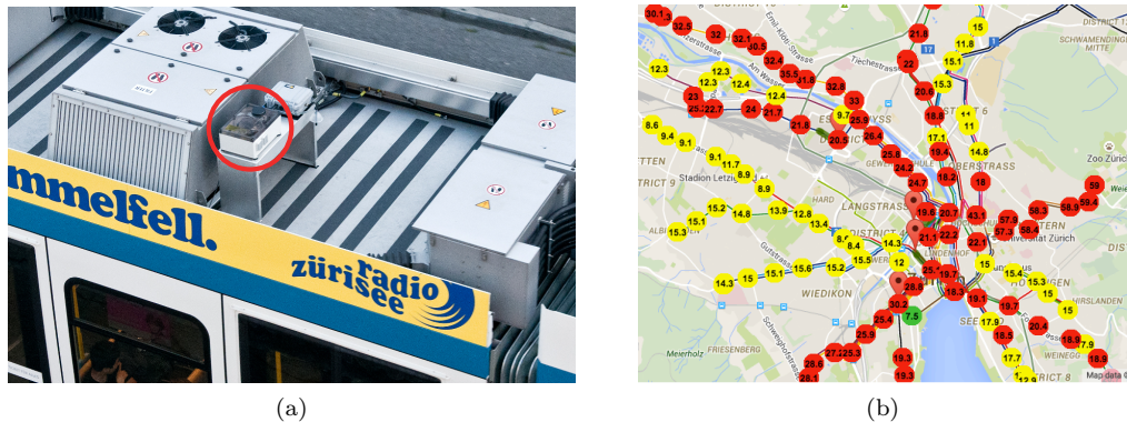
Figure 1.3: The Opensense [2] project using community-based sensing techniques to monitor air pollutions in the city of Zurich 1 . The sensor boxes (in the red circle in Figure 1.3a) are placed on public transportation vehicles for real-time monitoring. The captured Ozone levels are shown in Figure 1.3b.
