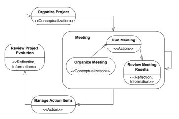
Figure 3. M.A.T. State Diagram
