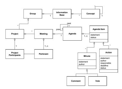
Figure 5. Conceptual model of M.A.T.
