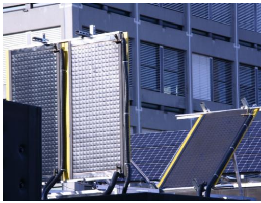
Figure 2: Experimental setup of the unglazed absorbers with different selectivity and inclination (left) and comparison of measured and simulated data of the outlet-temperature of the non-selective collector of \epsilon = 0.9 (right).
