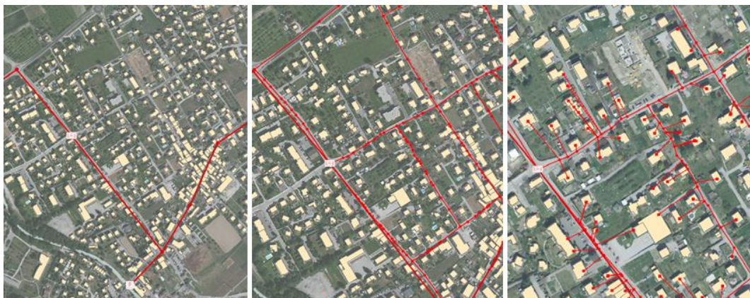
Figure 2: Concept for the three level network representations (from left to right: city, neighbourhood and street scale)
