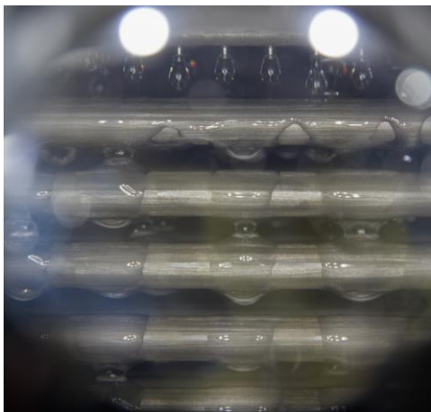
Figure 4: Picture of the tube bundle in the AD unit, showing the flow of sorbent (aqueous NaOH) over the tubes. Fine droplets group, reducing the wetted surface on the tubes.
