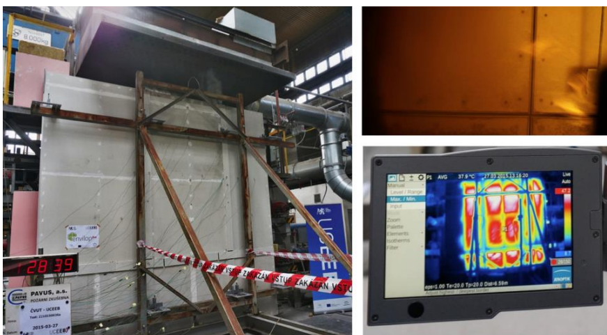
Figure 4: Testing of fire resistance EI(I<O) of EnvelopFIRE – laboratory setting, view into fire chamber after 90 minutes of experiment, and thermal monitoring of surface temperatures.
