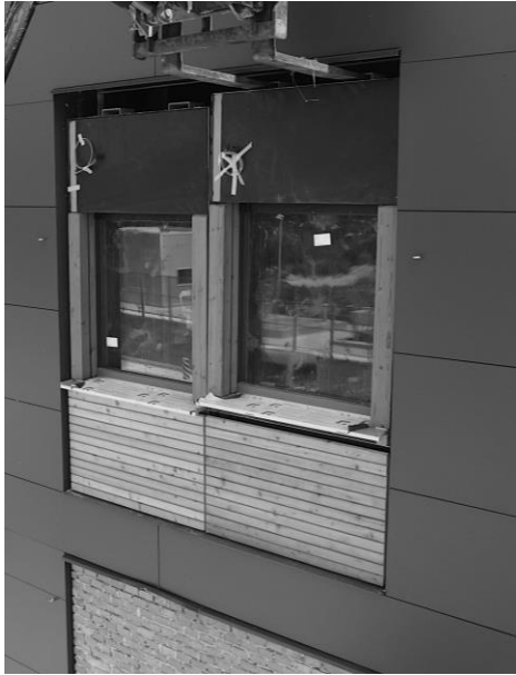
Figure 3: Long-term durability testing of the light bio-based envelope system. Left: Installation of four panels equipped with temperature sensors, relative humidity sensors and weight of moisture sensors embedded in panels and in modules' connections (measurement since November 2014). Right: Experimental setting of panels with various surface finishing (total area 48 m 2 , installation June 2015).
