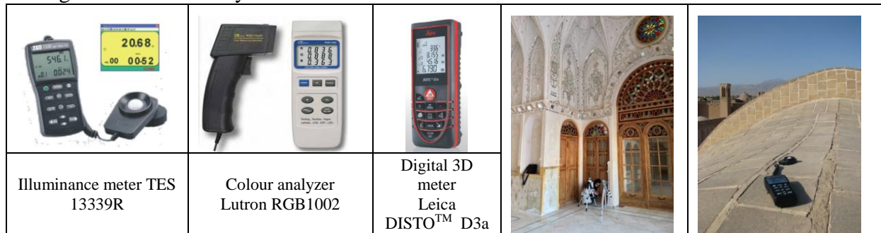
Figure 1: Field data collection instruments and location of the illuminance meters
