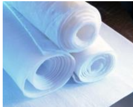
Figure 2: Aerogel Fibre Mat - Courtesy: Aspen Aerogel
