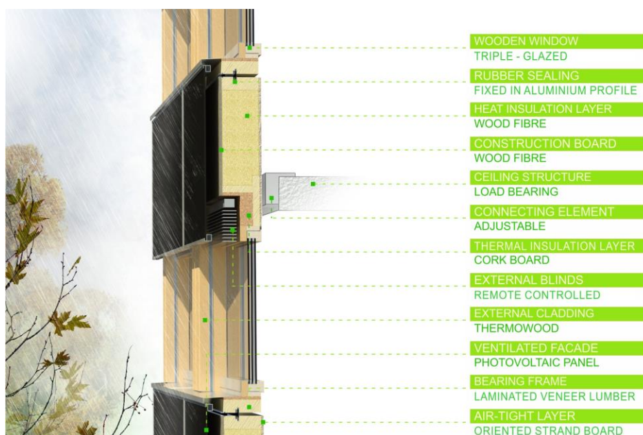
Figure 2: Typical composition of transparent panels.
