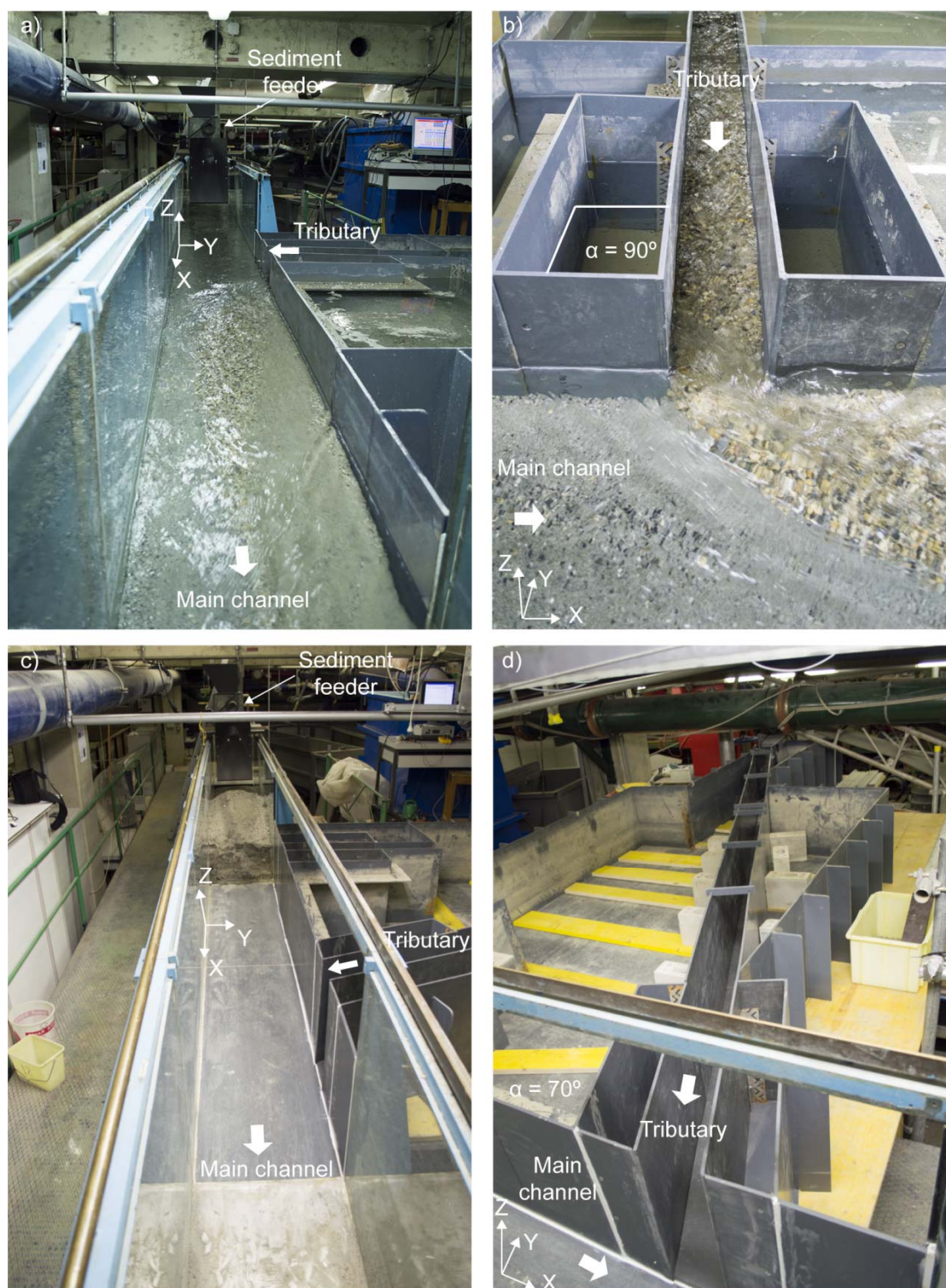
Figure 3.2 Experimental facility at LCH-EPFL. a) Upstream view of the main channel with \alpha = 90^\circ . b) Upstream view of the tributary with \alpha = 90^\circ . c) Upstream view of the main channel with \alpha = 70^\circ . d) Upstream view of the tributary with \alpha = 70^\circ .
