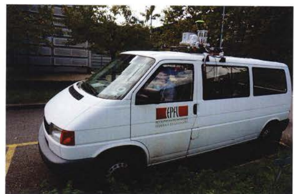
Fig. 1. Top: 'Gecko4Nav' housing the 4 MEMS IMUs; Middle: everything mounted on the support platform; Bottom: equipment mounted on a mini-van
