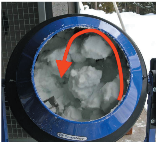
Figure 2. Granules in motion in rotating tumbler. One of the (two) mixing blades can be seen at the lower left corner.
