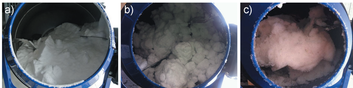
Figure 4. Snow inside tumbler for different experiments where (a) no persistent granules formed, (b) persistent-moist granules formed, and (c) persistent-wet granules formed.
