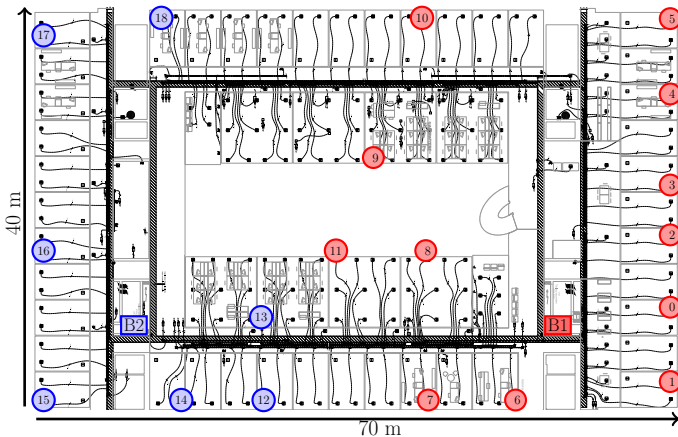
Figure 2: The electrical plan and the stations (0-18) of our testbed. There are two different PLC networks with CCo’s at stations 11 and 15. Stations marked with the same color belong to the same network and are connected to the same distribution board (either B1 or B2).
