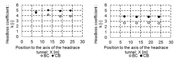
Figure 5 – Evolution of steady head losses as a function of the position in the connecting tunnel (X = 0 is the axis of the headrace tunnel) in both directions: (a) internal diameter of 1.55 m; (b) 1.69 m (Prototype scale).
