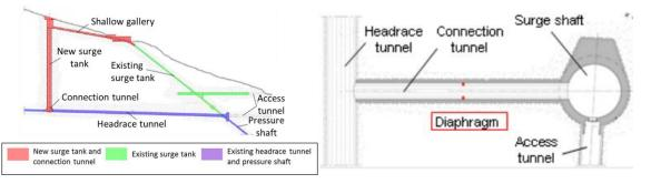
Figure 2 – (a) New vertical and existing surge tank (Hachem et al., 2013); (b) Plan view of the new (Hachem et al., 2013).
