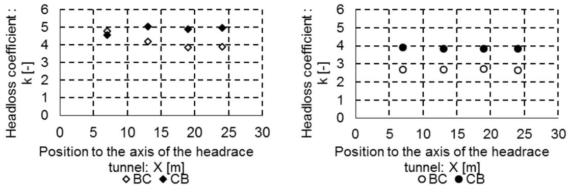
Figure 5 – Evolution of steady head losses as a function of the position in the connecting tunnel ( $X = 0$  is the axis of the headrace tunnel) in both directions: (a) internal diameter of 1.55 m; (b) 1.69 m (Prototype scale).
