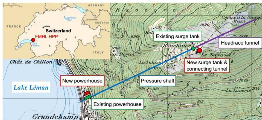
Figure 1 – Location of FMHL Pumped-storage plant and plan view of existing scheme and the new one (Hachem et al., 2013).
