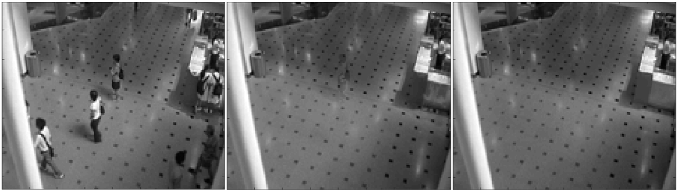
Figure 6: One frame of the recovered background from a video of a shopping mall lobby. left) actual frame, middle) recovered low-rank background using Robust PCA and right) recovered background using our proposed model. The presence of graph in our model enables better recovery and removes all the walking people from the frame.
