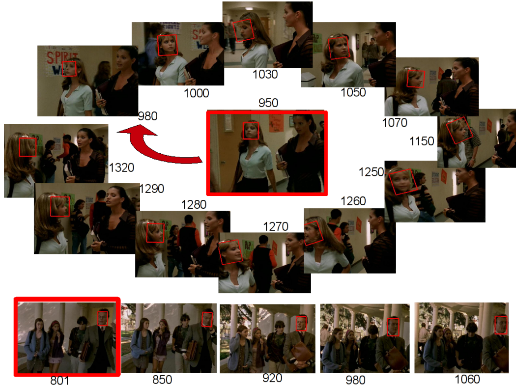
Figure 7. Tracking while the person is moving. The number accompanying each picture is the corresponding frame No. The red window indicates the starting frame. The red boxes in the following frames show the template boxes estimated by the algorithm.
