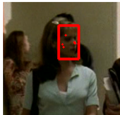
Figure 8. Example of a profile face instance with a small number of invariant features indicated by the red points.
