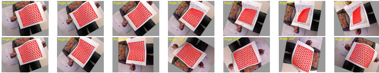
Figure 9. Tracking a rotating deformable surface. Top row: Without rotation handling, tracking with the original GBDF descriptors eventually breaks down. Bottom row: Our modified GBDF features can track the whole sequence with up to 360^\circ of rotation.
