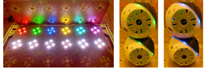
Fig. 8. LED illumination. (a): Grid tiles. (b), (c): Roombots modules. (a) Grid colors in full intensity. Top: red, green, blue, yellow, cyan, violet tiles. Bottom: 6 white tiles. (b) Module in green. (c) Module in blue.
