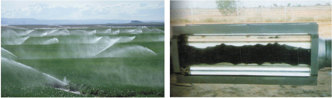
Figure 1 – Examples of co-axial flow. On the left agricultural irrigation, reprinted from Eggers & Villermaux (2008). On the right lubricated pipeline for the oil transportation (INTEVEP, SA).
