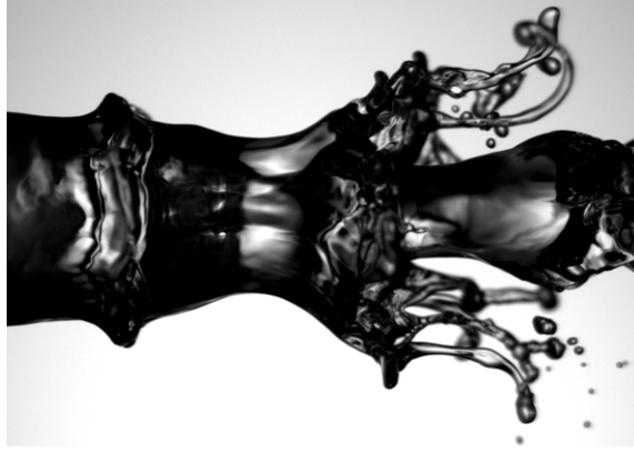
Figure 5 – Typical destabilization of a slow water jet u_{water} = 0.6m/s by a fast coaxial air stream u_{air} = 35m/s . The primary instability forms ligament which are subsequently broken into droplets. Experiment performed by from Marmottant & Villermaux (2004)
