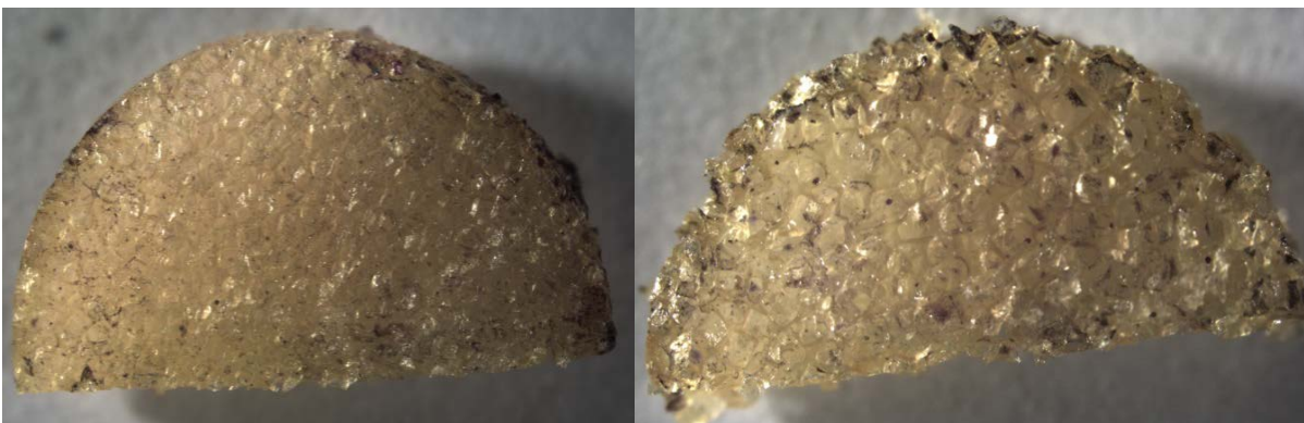
Figure 21: Surface of two scaffold seeded with 40% strains and 5 mm/s unloading velocity. The left scaffold being polymerized using fine particles and the right one using rough ones. The black points are the MTT stained cells.
