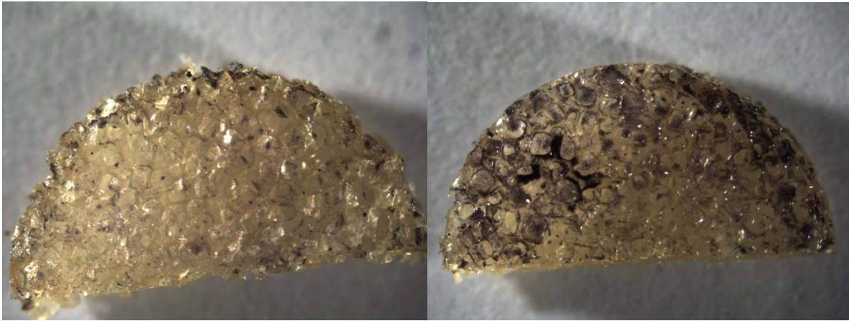
Figure 20: Surface of two scaffolds of rough particles seeded with 40% strains and 5mm/s unloading velocity for the one in the left and 0.1mm/s unloading velocity on the right(The black clusters mean cell are just in the surface).
