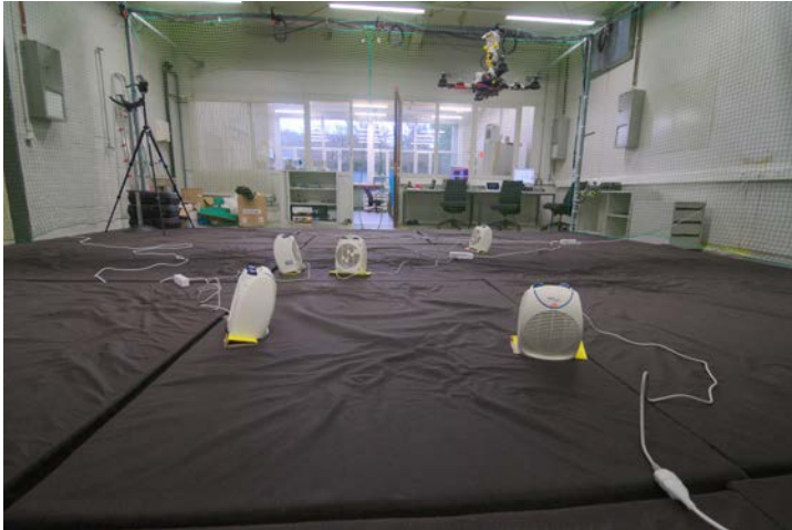
Figure 9.2 – Experiment in progress. Electrical heaters on the ground produce a surface temperature gradient to be estimated by the quadrotor.
