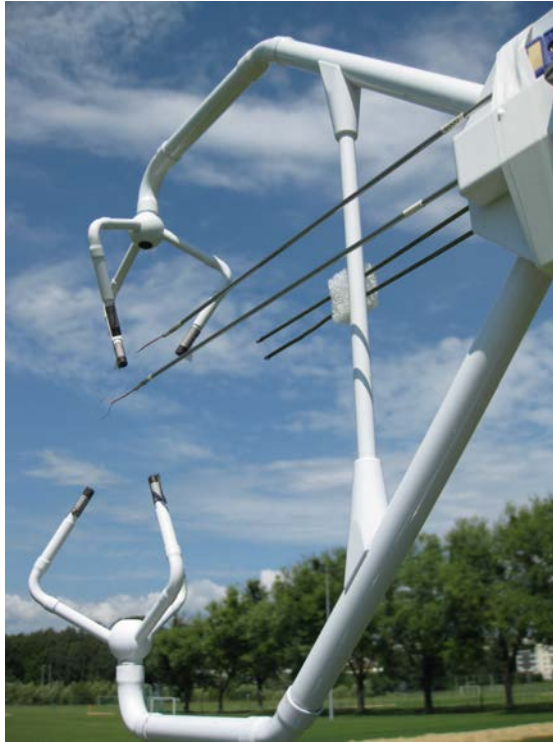
Figure 5.2 – Reference deployment setup. Sonic anemometer deployed in an open, grass-covered field, with the NTC extending into its sample volume on a probe.
