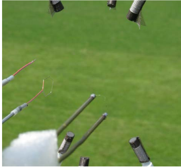
Figure 5.3 – Close-up of sonic anemometer's sample volume. The anemometer's transducers are visible along the top and bottom of the photo, and the NTC is visible in the center.
