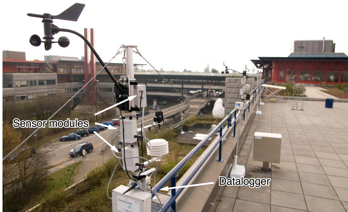
Figure 3.1 – Sensorscope station on the rooftop of EPFL's GR building.
