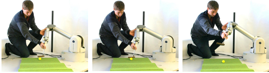
Figure 2.2: An example of kinesthetic teaching. The robot is gravity compensated, allowing the teacher to effortlessly guide it through the motion.
