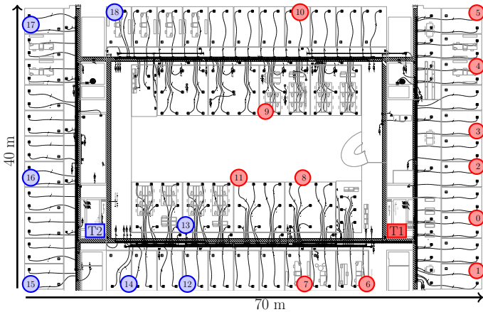
Figure 1: The electrical plan and the stations (0-18) of our testbed. There are two different PLC networks with CCo’s at stations 11 and 15. Stations marked with the same color belong to the same network and are connected to the same electrical table (either T1 or T2).
