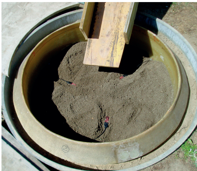
Figure B.1: Installation of the FDR probes in the lysimeter, upper depth (25 cm).
