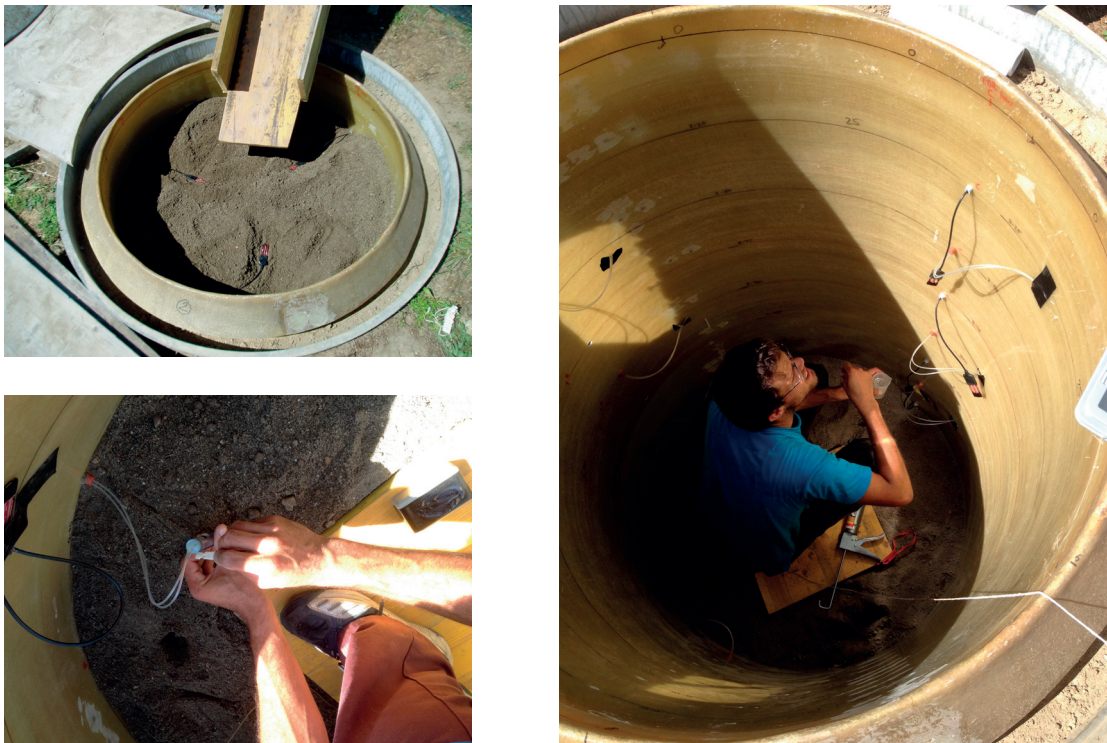
Figure A.2: Filling and instrumentation of the lysimeter. The FDR probes and porous cups monitored depths can be seen on the right. Filling state and top-depth FDR probes before the planting of the willow (top left). The porous cups were sealed with epoxy resin (bottom left).
